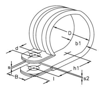
$\begin{array}{lll} \text{b1} & = 25.0 \\ \text{d} & = 8.4 \\ \text{Diameter D} = 28 \\ \text{h1} & = 28.5 \\ \text{I} & = 8.5 \\ \text{s} & = 1.00 \\ \text{s2} & = 2.0 \\ \text{Width B} & = 20 \\ \end{array}$
